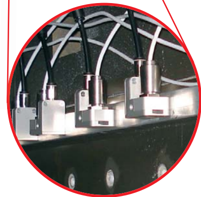
Small optris CT LT sensing heads installed in a machinery with a laminar air purge collar.
